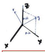
Orientation Vector: target.O.Y = 0.5 target.O.Z = 0.5
