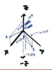
Normal Vector: target.N.X = 0.707 target.N.Z = 0.293
