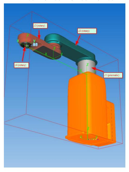
Below is a detailed kinematic structure and break down structure of the robot for solving the inverse kinematic problem.
